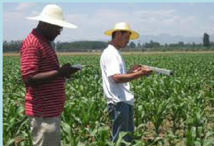
Line quantum sensors measuring canopy cover for transpiration estimation
